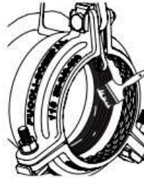
5. Lubricate the lip seal ring and pipe. Don't use oil
